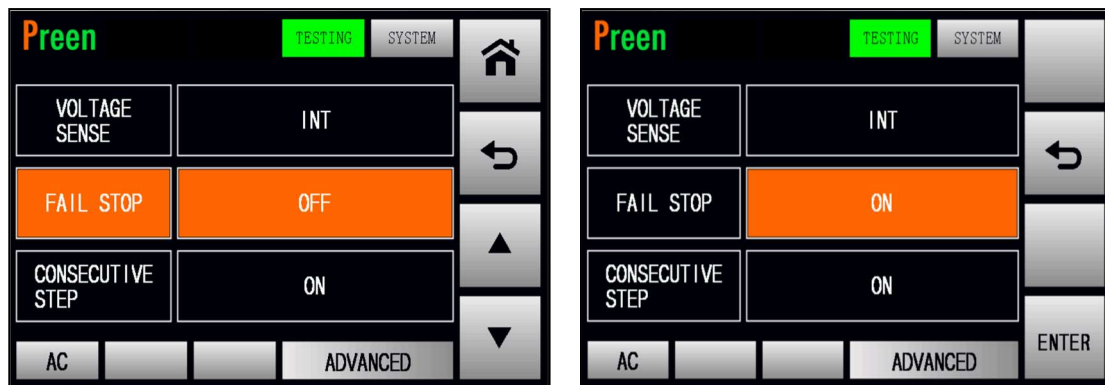
Figure 3.21 Enable the fail stop feature (ADVANCED mode)
