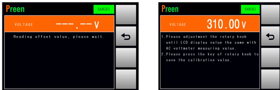
Figure 4.6 Enable the calibration of the HI-Range voltage 310V
