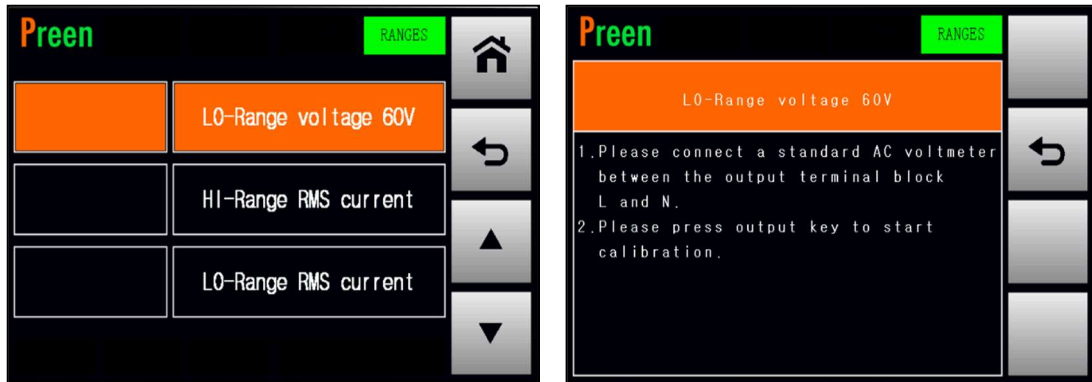
Figure 4.11 Enter into the page which calibrates the LO-Range voltage 60V
