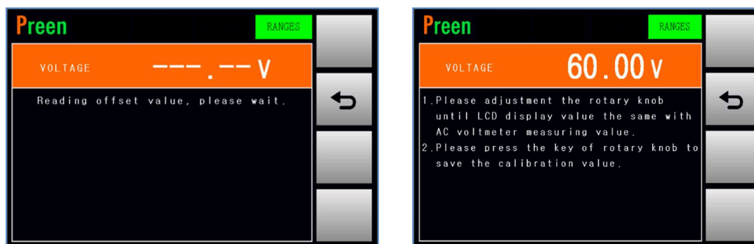
Figure 4.10 Enable the calibration of the HI-Range voltage 60V
