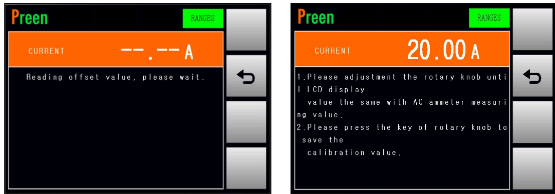
Figure 4.20 Enable the calibration of the output socket current
