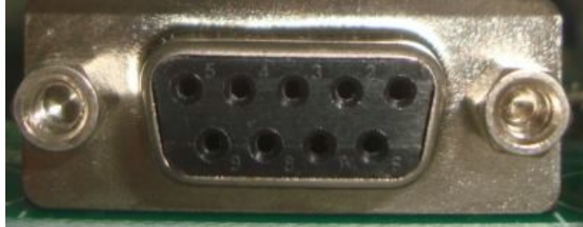
Fig. 5-12 Diagram of RS485 port
