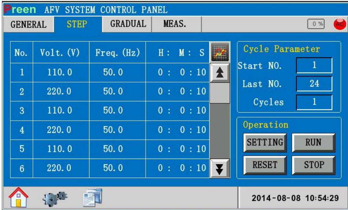
Fig. 5-5(a) Step mode setting interface
