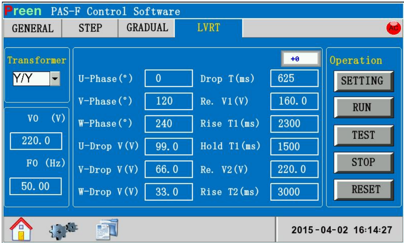
Fig. 4-7 LVRT setup menu
