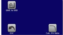
This table function uses the standard XY generator to let the power supply simulate solar panels or solar cells with certain characteristics. The device calculates an IU table from four typical values. While the function is running, the user can adjust a parameter "Irradiance" between 0% (darkness) and 100% (bright light) in 1% steps to simulate different light situations.
