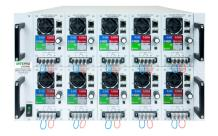
Tustin, CA— March 23, 2016—<u>Intepro Systems</u> announces the ELR 5000 modular, programmable DC load—the latest addition to the Intepro family of power system automatic test equipment (ATE). Housed in a 6U, 19" rack enclosure, the ELR 5000 can accommodate up to 10 completely self-contained, fullyprogrammable DC load modules with 320W nominal power, each. The modules can be used separately or in parallel, providing up to 3200 Watts. Up to 93% of the load power is
