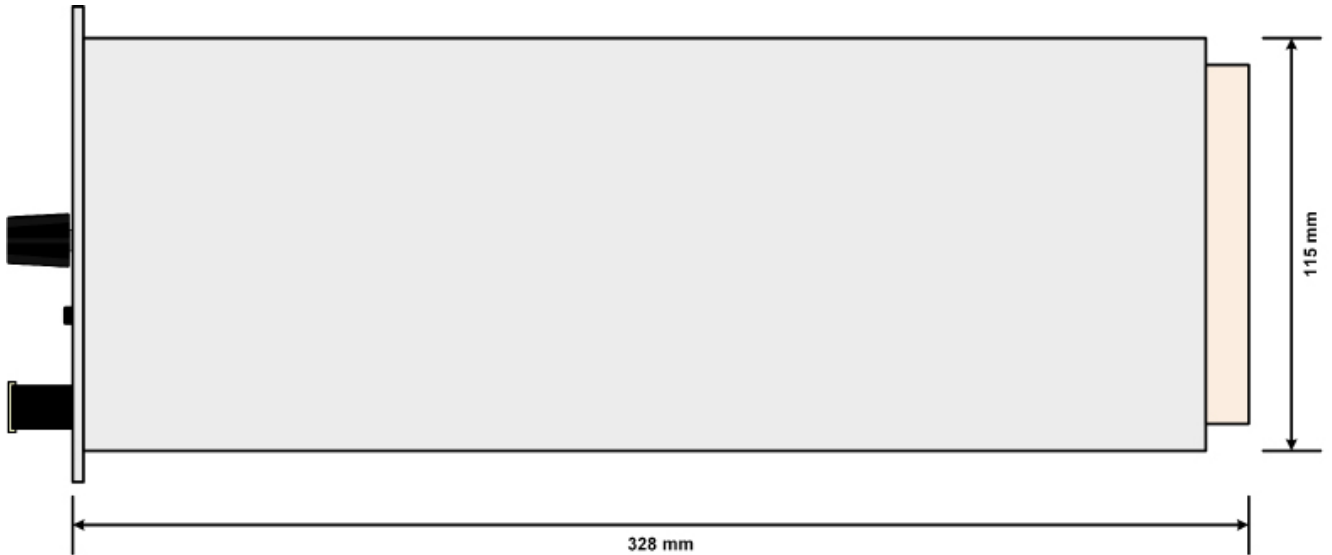
Figure 6 - Side view of load module
