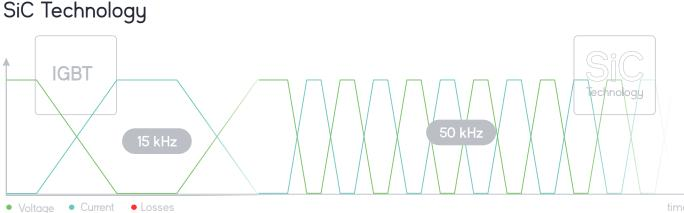
Transitioning to SiC technology results in an increased switching frequency of the converter, which translates into higher dynamics, faster transients and enhanced performance, making it the perfect candidate for EoL environments, R+D, Validation and Power Hardware in The Loop (PHiL) testing.
