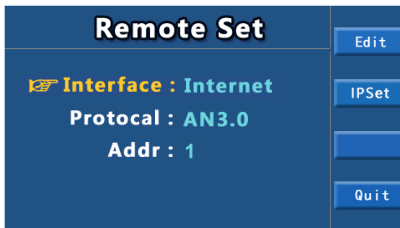
Figure 3.2.11 LAN port power supply setting
