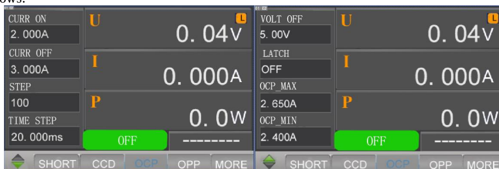
Figure 4-25 Overcurrent mode standby
