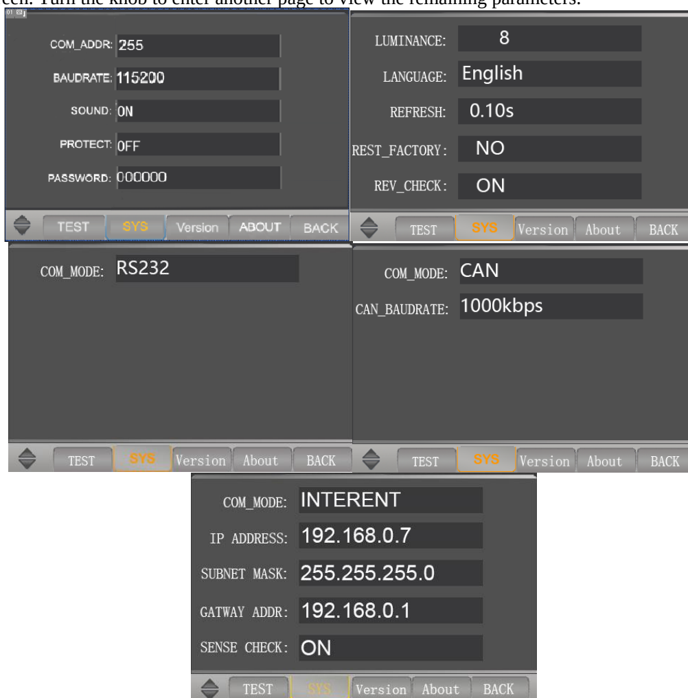
Figure 4-34 System Setting System Settings parameters and meanings:
