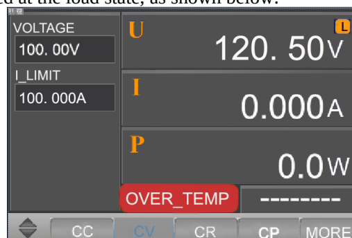
Figure 5-4 Over temperature enters the interface
