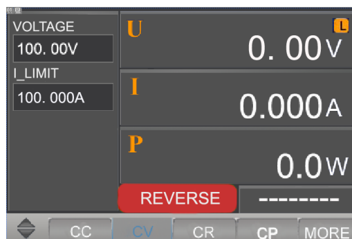
Figure 5-5 Reverse alarm interface
